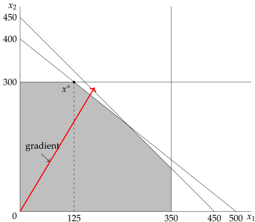
Figure 4.1: Feasible region and objective direction of Example 4.4
